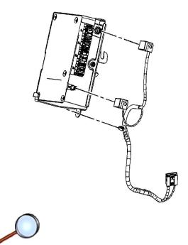
4. Disconnect the VCIM electrical connectors as necessary.
